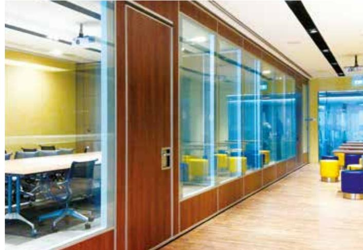
Acoustic operable glasswall maintains the aesthetic appeal of glass while providing acoustic separation to STC 44. Acoustic operable glasswalls are available as single and paired panels only. They consist of glass surrounded with an aluminum frame that is nominal 83mm thick. Each panel has a 25mm clearance bottom retractable seal that exerts downward force. The standard aluminum frame finish is clear anodized but it may also be ordered powder coated or custom anodized.
